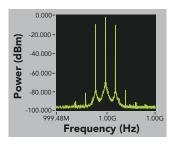
By taking more samples over a longer time, you can decrease the resolution bandwidth and separate nearby signals from one another. The better resolution comes at the cost of longer processing times, though. mines the frequency range or the bandwidth. The number of sampled points determine the frequency resolution, also called the resolution bandwidth (RBW).
