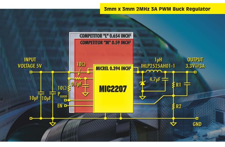
Micrel'S MIC2207 is a high efficiency PWM buck (step-down) regulator that provides up to 3A of output current. The MIC2207 operates at 2MHz and has proprietary internal compensation that allows a closed loop bandwidth of over 200KHz.
