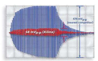
Design Example: 1.5 volt LVCMOS 4mA, I/O, 100 aggressors shown.
