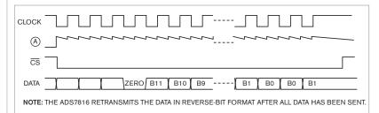
Figure 2 An SPI-clock waveform (top trace) evokes data (bottom trace), and peak detection of the clock (the waveform at Point A in Figure 1) yields a signal (next-to-bottom trace) that mimics the chip-selection line's behavior.
