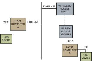
Figure 2 USB-interface adapters extend the interface capabilities for host computers; they do not extend the interface capabilities for other USB devices.
