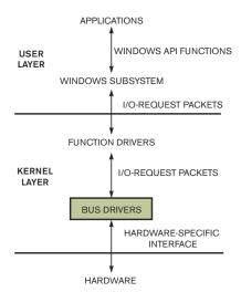
Figure 3 New bus drivers replace the USB/PCI drivers to provide the USB/ network capability for the USB-system software on the host computer and the USB server.
