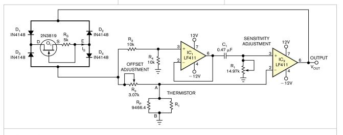
Figure 1 This simple circuit linearizes a thermistor's response and produces an output period that's proportional to temperature.
