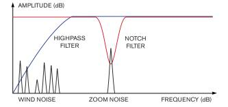
Figure 2 Digital filtering can suppress noise that is limited to one part of the audio spectrum, such as low-frequency wind noise and narrowband zoom noise.
