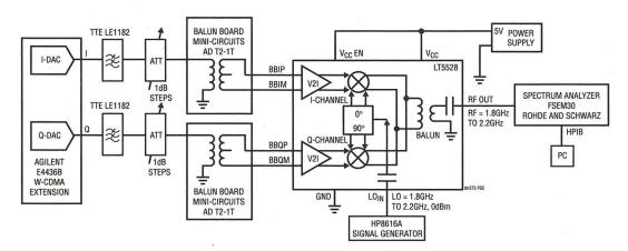
Figure 2. ACPR Measurement Setup
