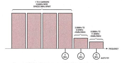
Figure 1. WCDMA ACPR Limits, Per 3GPP TS 25.104, Section 6.6.2.2.1
