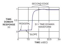
Figure 1 Data following the second edge is a mixture of gain and impedance information.
