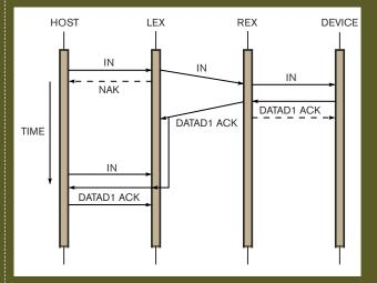
Figure B This diagram shows the NAK and ACK (acknowledge) signal sequence for a USB transaction over the wireless interface (courtesy Icron).
