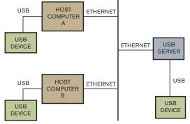
Figure 1 The USB server acts as a host controller to a USB device and coordinates with each host/client to enumerate the USB device on each host computer.
