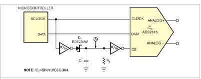
Figure 1 Two inverters and a few components can substitute for an SPI ADC's chip-select line.
