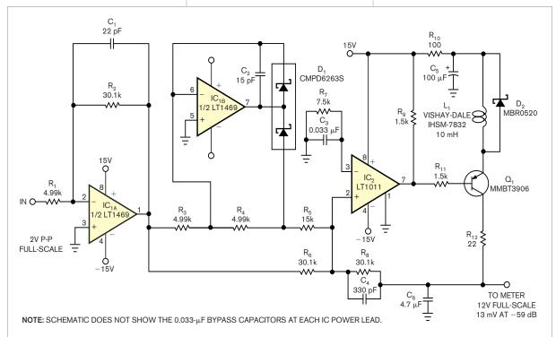
Figure 1 This inductor-compensated voltage-unit meter displays a 60-dB dynamic range.
