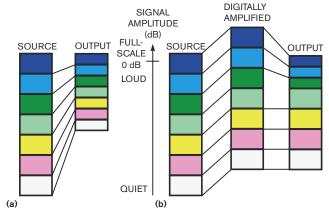
Figure 3 Using dynamic compression (a) or peak limiting (b) coaxes more volume from small speakers.
