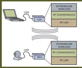
Figure A The Lex and Rex dongles comprise three layers. The top layer is the ExtremeUSB protocol layer, which compensates for the effects of delay. The RF-convergence layer formats USB packets in a manner that is more suitable for transmission over RF (courtesy Icron).
