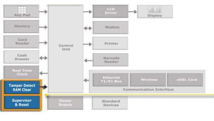
ST products for Point of Sales applications range from dedicated MCUs through state-of-the-art discretes to give you the widest design options. And now with the STM1403 and STM1404, the world's first security supervisors with FIPS levels 3 and 4 attack detection, we're making your design task even easier.
