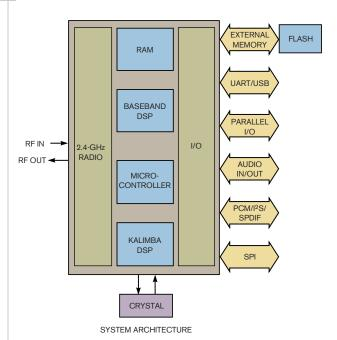
Packing more power, performance, and features into an 8×8-mm BGA, the BlueCore-5 multimedia external IC extends data rates and adds multimedia support.
