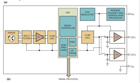
The reality-tolerant, multisensor Melexis MLX90316 Hall-effect sensor has 360° rotary positions. It includes a flux concentrator above the passivation layer.
