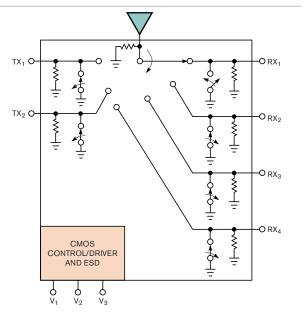
Switch your RF path among six ports, with the nearly RF-transparent SP6T CMOS switch, which meets the stringent mandates of GSM/WCDMA applications.
